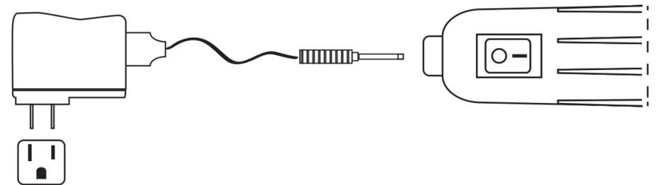
2. When charging with DC adapter, insert the battery charger plug into the charging port on the worklight and the other end into a standard 12-volt DC outlet.
